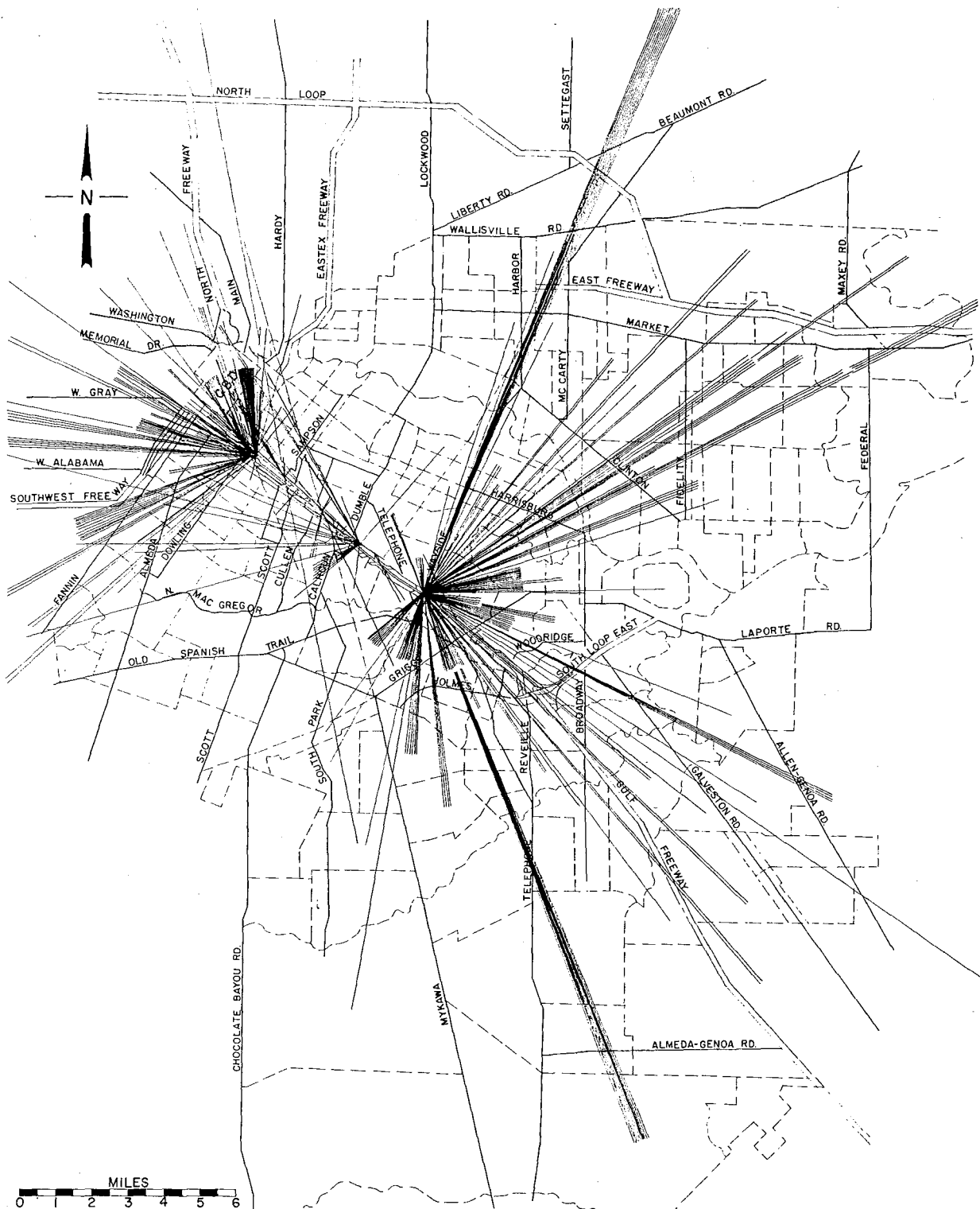
WAYSIDE ENTRANCE RAMP AREA OF INFLUENCE ORIGIN-DESTINATION DESIRE LINES VIA FREEWAY LINK 6:45 - 8:30 A.M.
