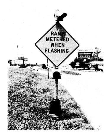
FIGURE 1. RAMP SIGNAL AND ADVANCE WARNING SIGN.
