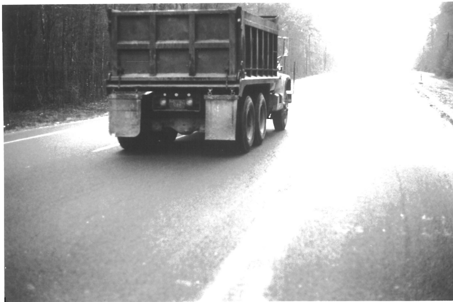
Figure 20. Splash and Spray Behind Truck in 0.05 in/h Rainfall K_{avg} = 0.07 ; Location: 87/3057/L&R
