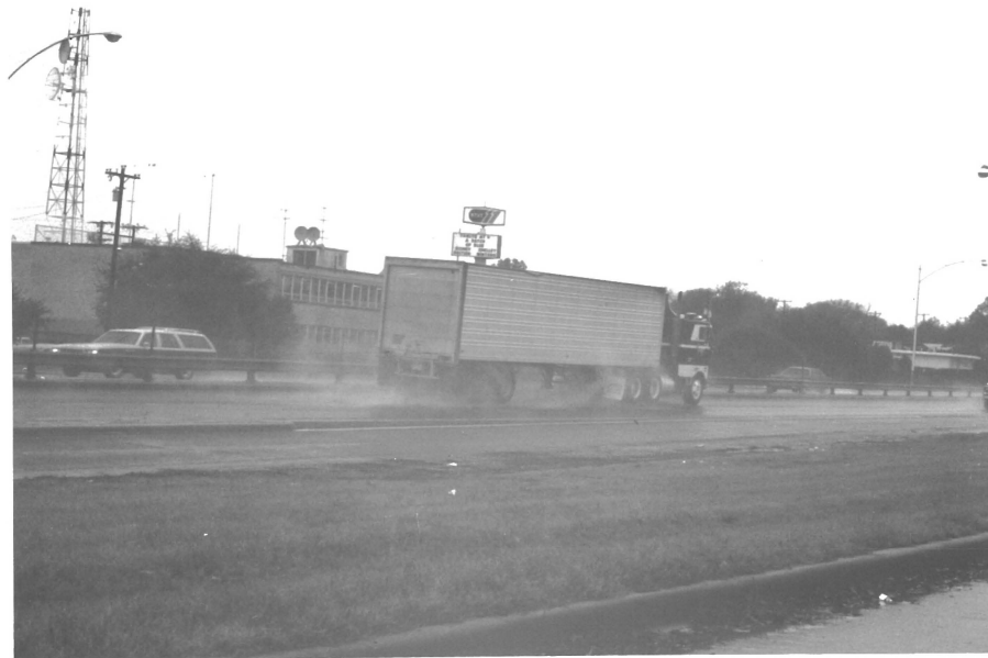
Figure 13. Splash and Spray Behind Truck in 0.04 in/h Rainfall K_{avg} = 0.014 ; Location: 30/1681/R&S
