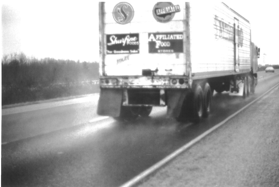
Figure 16. Splash and Spray Behind Truck in 0.25 in/h Rainfall K_{avg} = 0.15 ; Location: 10/7392/L 2/9/78
