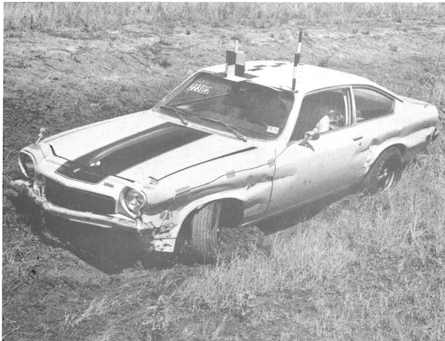
Figure 16. Vehicle before and after Crash Test 2. (93 km/hr and 14 degree impact angle)
