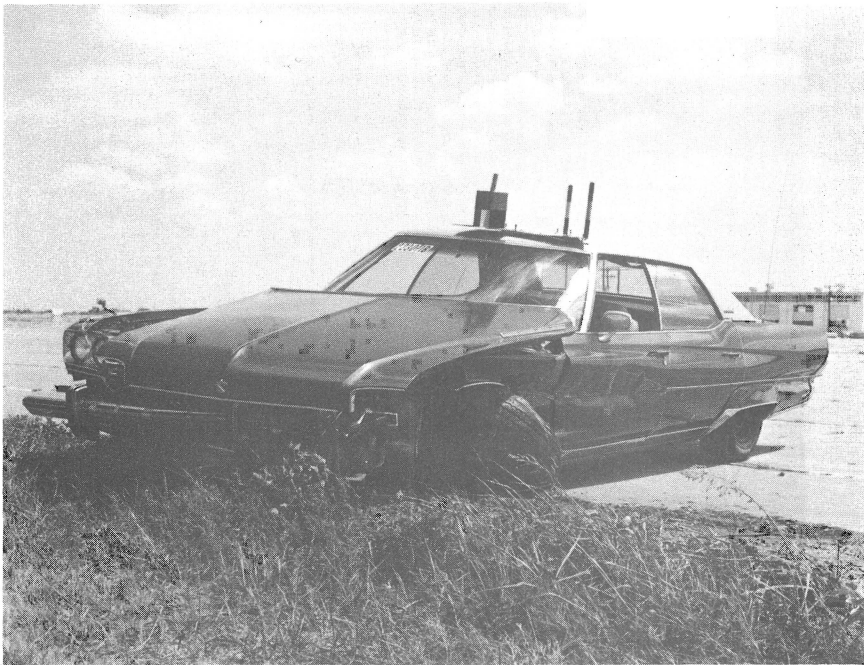
Figure 12. Vehicle before and after Crash Test 1B on TUBULAR W-BEAM Bridge Rail - 99 km/hr, 27.5°.
