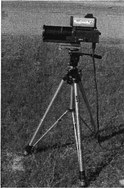
Figure C-1. Traffic Management System Lidar and Camera.
