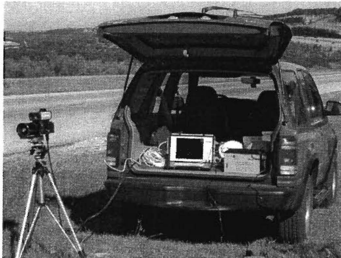
Figure C-5. Typical TMS Setup.
