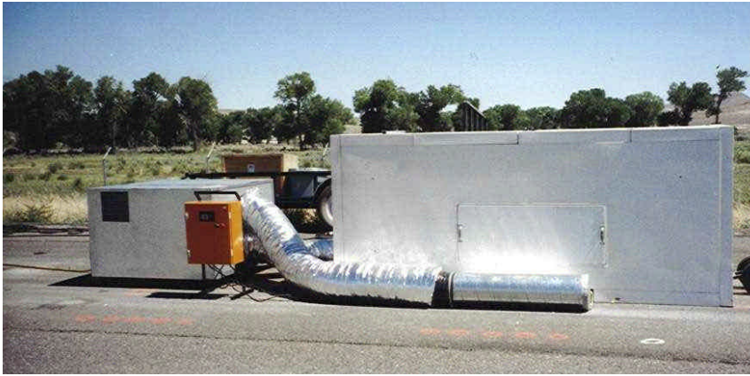
Figure 2. MMLS3 at WesTrack inside environmental chamber
