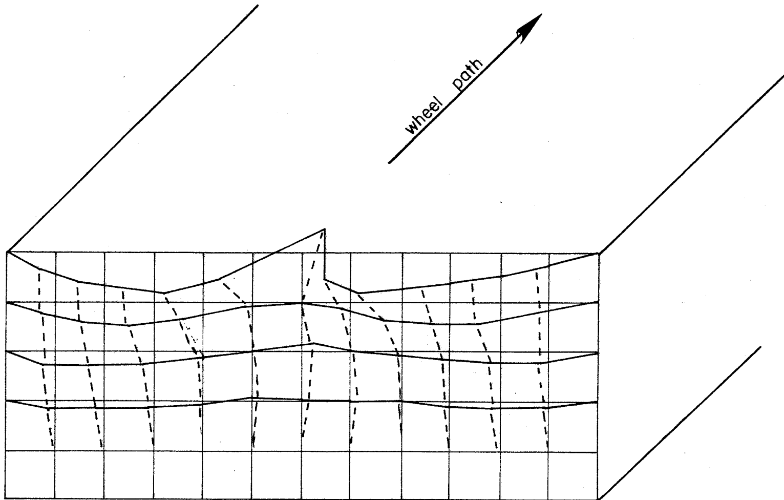
Figure 10. Residual longitudinal movement distribution after the first pass of a 200-pound load with a 100 p.s.i. contact pressure.
