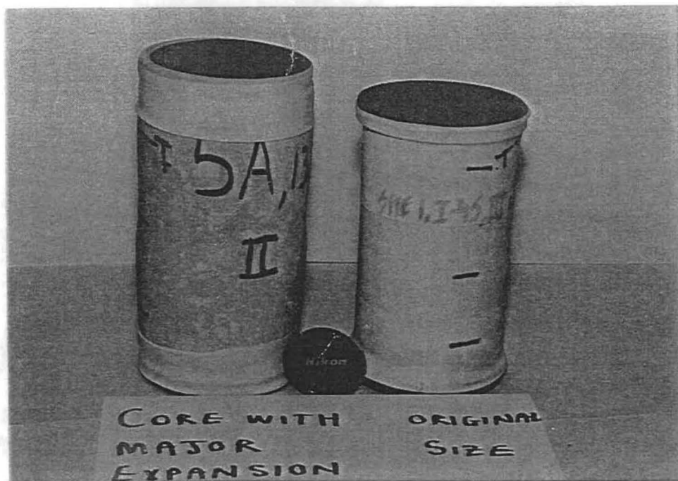
Figure 16. Two Soil Samples with 0.8% Sulfates. Sample on the Left Contains 6% Lime and Expanded 6% More than the Sample on the Right Which Contains No Lime.
