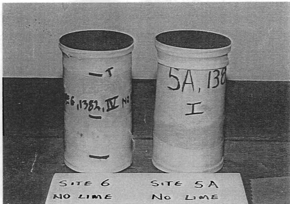
Figure 14. Expansion of Samples Containing No Lime. Sample on Left Contains Less than 0.2% Sulfates and Sample on Right 0.8% Sulfates.
