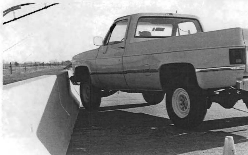
Figure 39. Vehicle/barrier geometrics (test 1959A-5).
