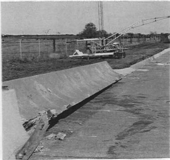
Figure 22. Post test damage to limited slip concrete barrier connection installation (1959A-2).
