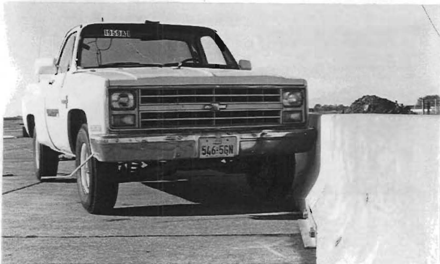
Figure 12. Vehicle/barrier geometrics (test 1959A-1).
