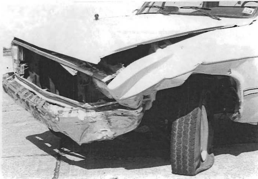
Figure 43. Post test damage to vehicle (1959A-5).
