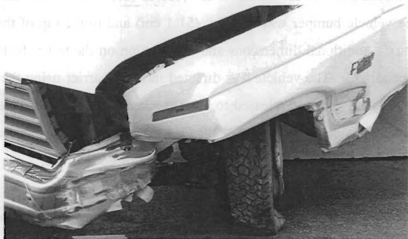
Figure 37. Post test damage to vehicle (1959A-4).
