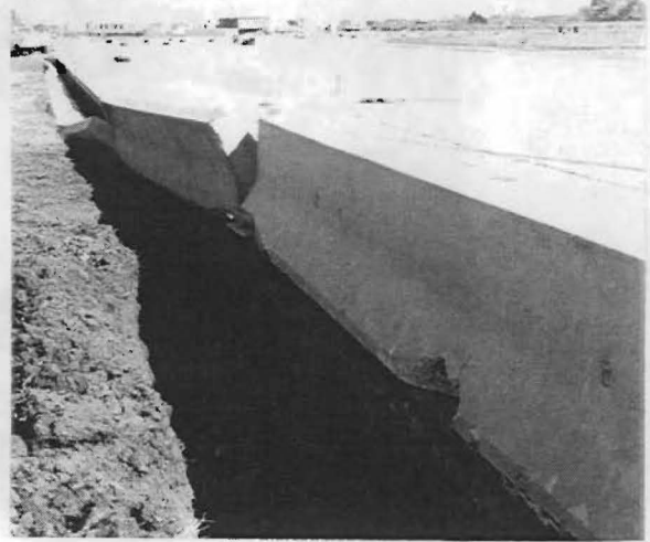
Figure 22. Post test damage to limited slip concrete barrier connection installation (1959A-2).
