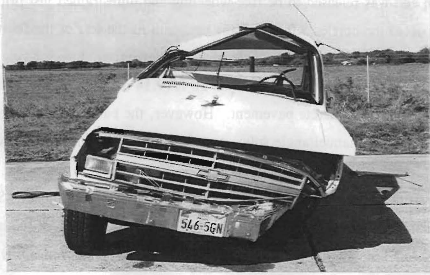
Figure 17. Post test damage to vehicle (test 1959A-1).
