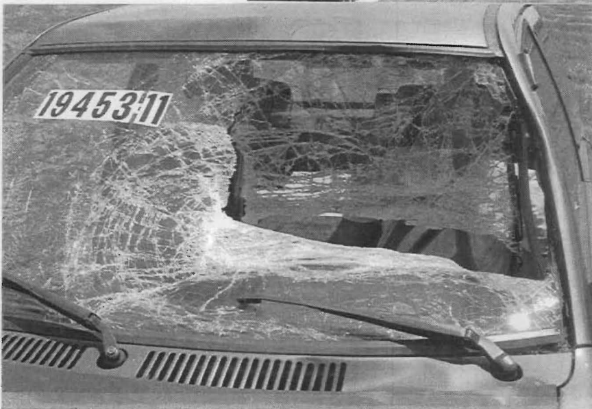
Figure M-9. Details of occupant compartment intrusion after test 19543-11.
