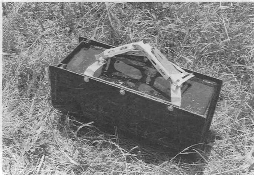
Figure M-7. Mailbox installation after test 19453-11.
