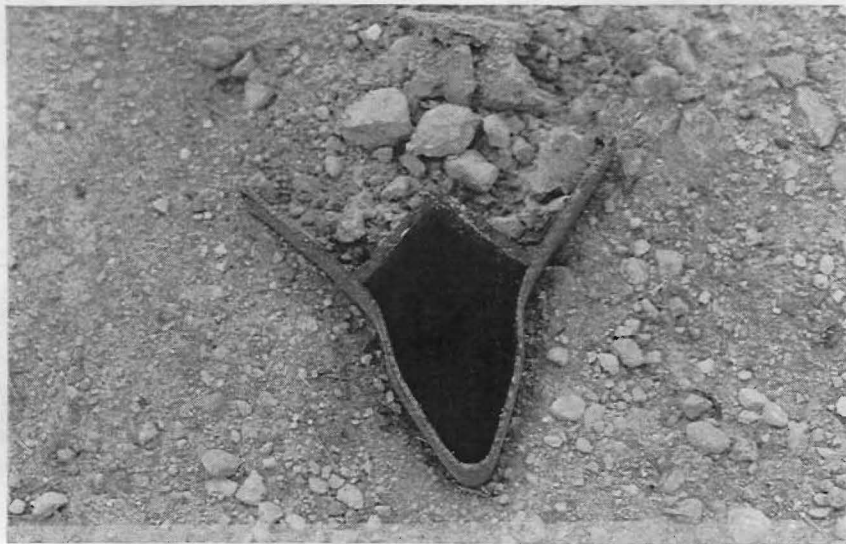
Figure I-7. Mailbox/support and base after test 19452-7.
