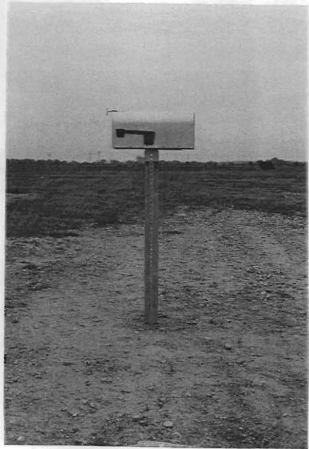
Figure C-1. Mailbox installation for test 19452-1.
