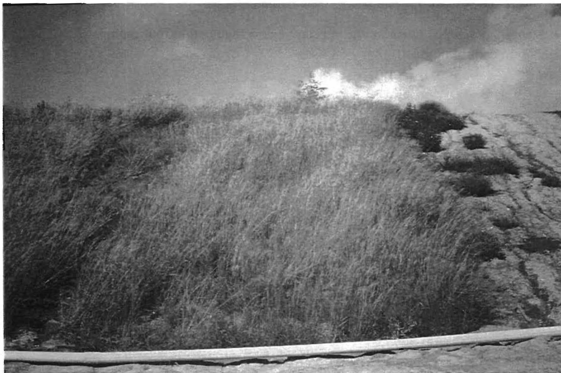
Figure 43. Vegetative coverage on a 3:1 Clay Straw product plot
