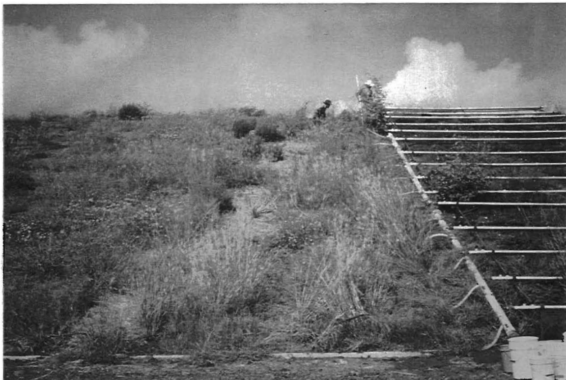
Figure 44. Vegetative coverage on a 3:1 Clay Excelsior product plot
