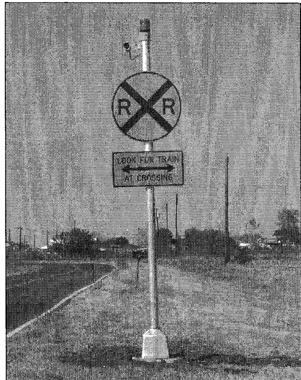
Figure 1-2. LOOK FOR TRAIN AT CROSSING Enhanced Sign System.
