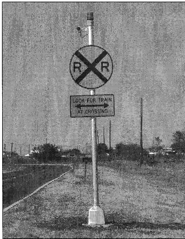
Figure 2-4. LOOK FOR TRAIN AT CROSSING Enhanced Sign System with Flashing Strobe.
