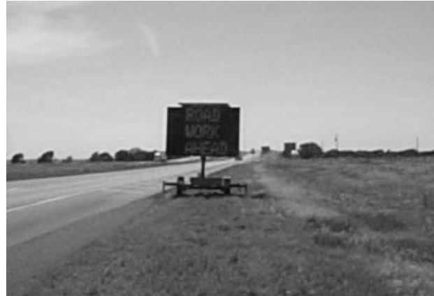
Figure 41. Portable Variable Message Sign.
