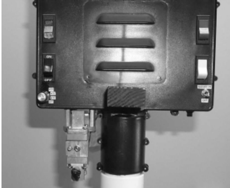
Figure 16. Flagger Paddle Controls.
