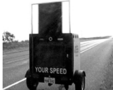
Figure 46. Speed Display Trailer.
