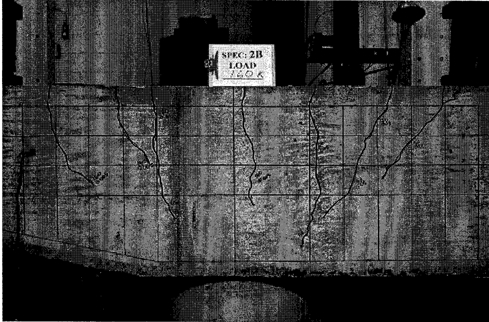
Figure 4.2. Typical Laboratory Observed Cracking Pattern of Group #1 Specimens at P = 160 Kips.
