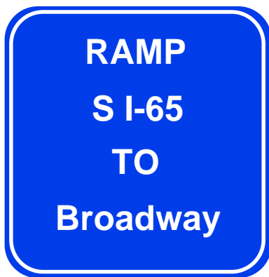
Figure 7-4. Ramp Marker Design.
