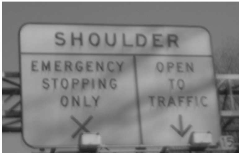
Figure 5-2. Explanatory Sign Used for Shoulder/Lane.
