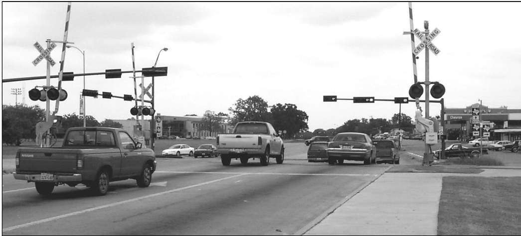
Figure 2. Signalized At-Grade Intersection Near Highway-Railroad Grade Crossing.
