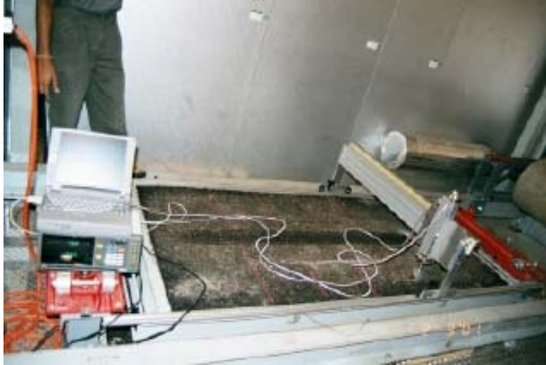
Figure 14. Profilometer Used to Measure MMLS3 Rut Depth.
