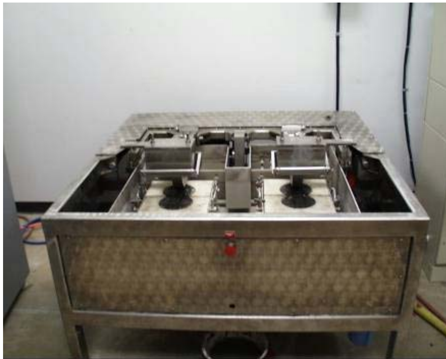
Figure 16. HWTD Loaded with Specimens.
