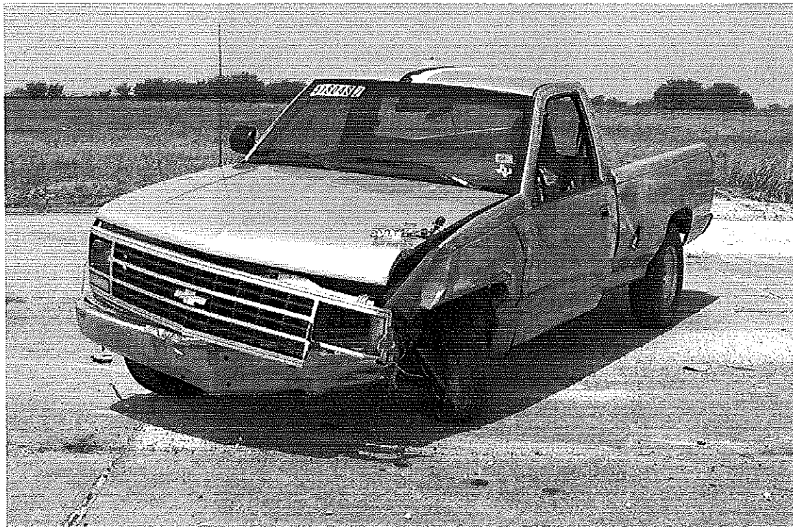
After being uprighted Figure 11. Vehicle after Test 418048-2
