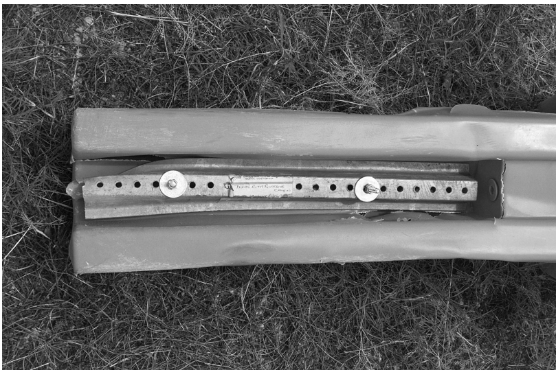
Figure 17. Step 2 Mailbox on Steel U-Channel after Test 417921-3.
