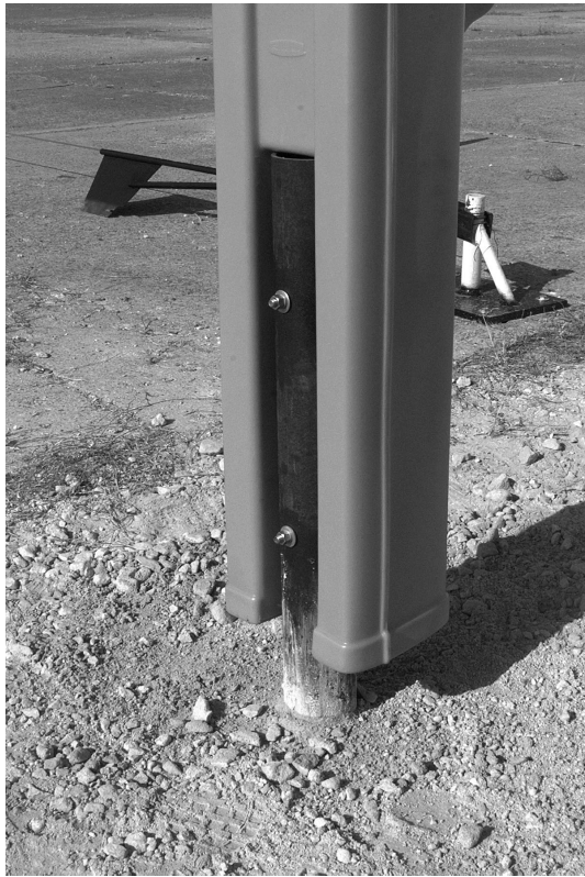
Figure 6. Rubbermaid Mailbox on Steel Pipe Post before Test 417921-4.
