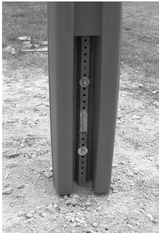
Figure 4. Step 2 Mailbox on Steel U-Channel before Test 417921-3.
