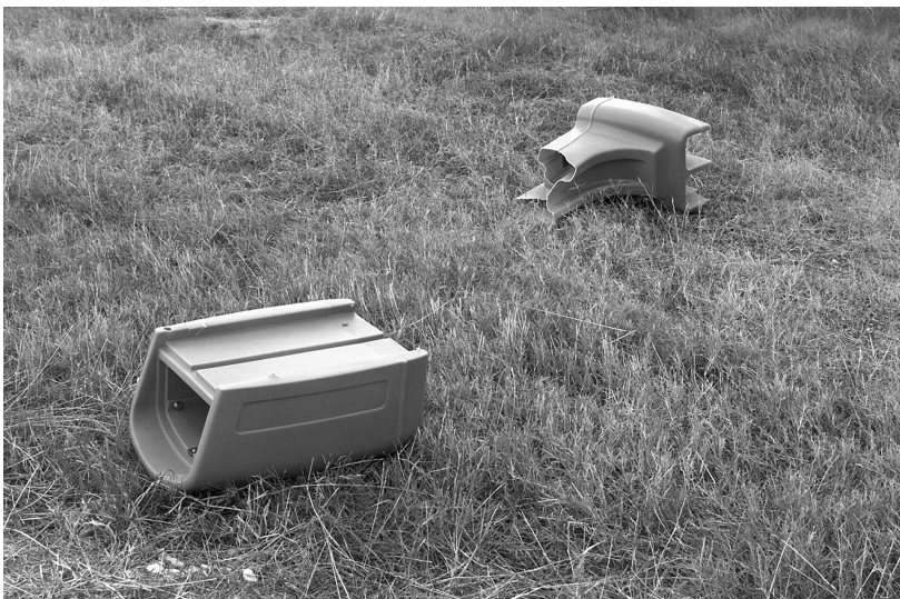
Figure 10. Step 2 Mailbox on Timber Post after Test 417921-2.
