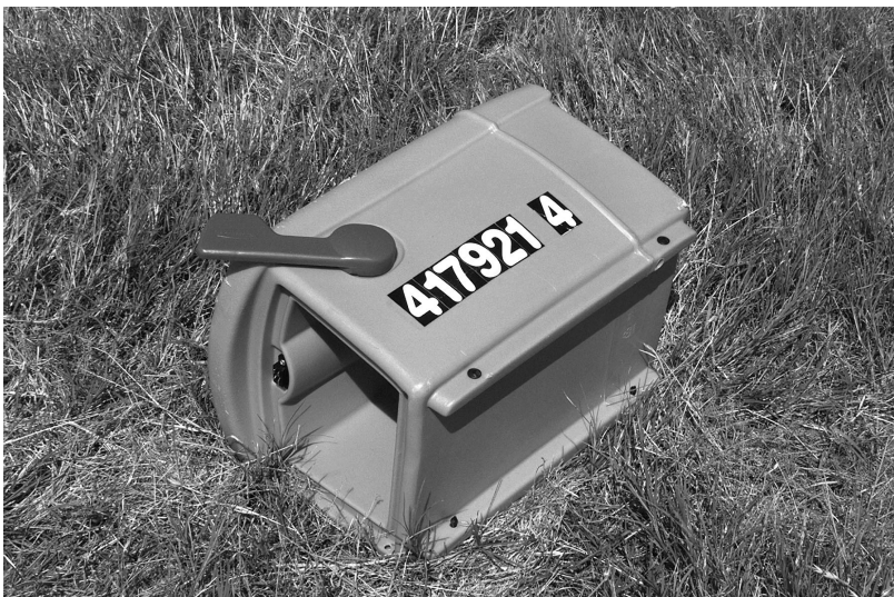
Figure 24. Rubbermaid Mailbox on Steel Pipe after Test 417921-4.
