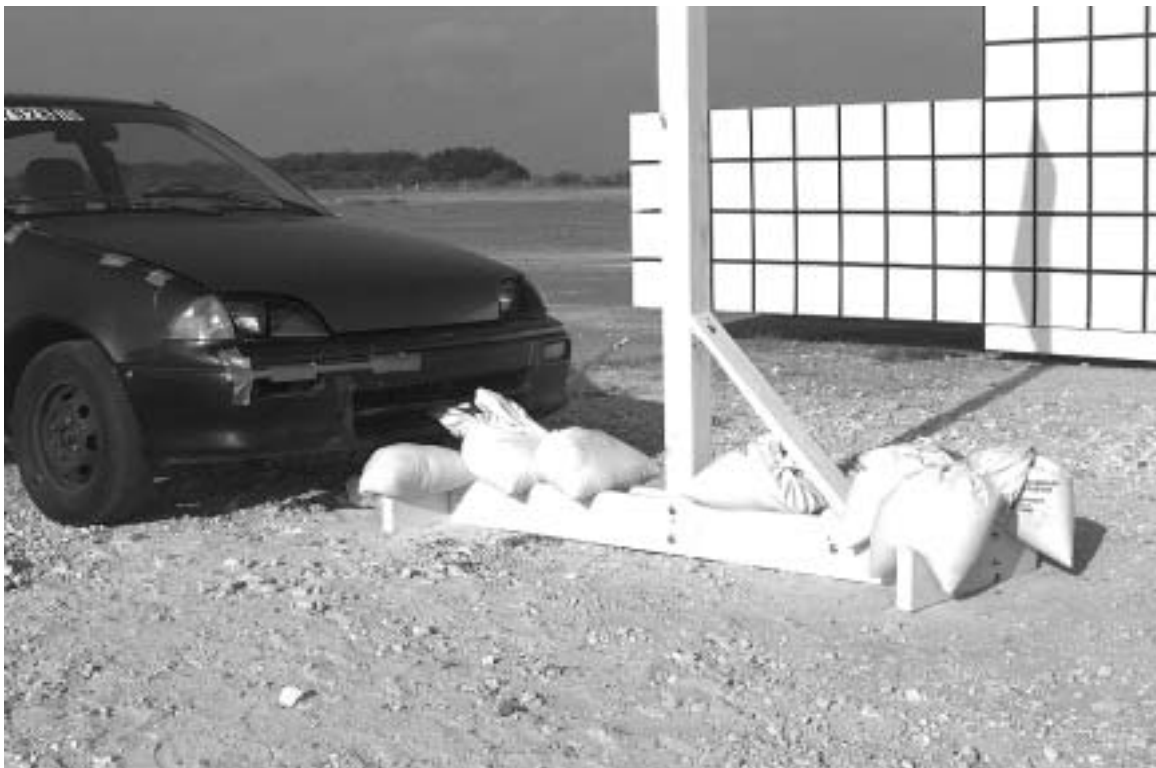
Figure 97. Vehicle/Installation Geometrics for Test 417928-10.
