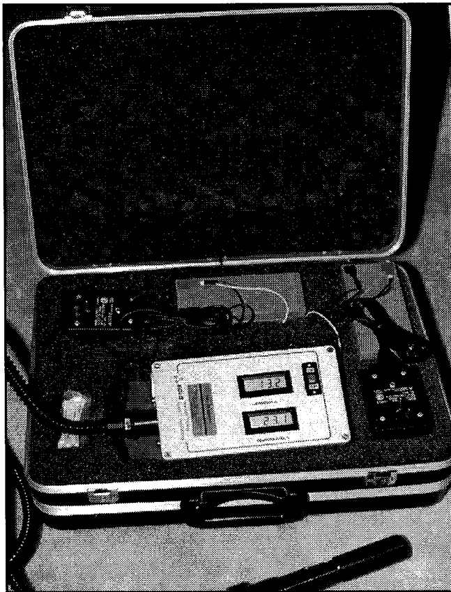
Figure 3.22 View of the Dew Point Indicator.
