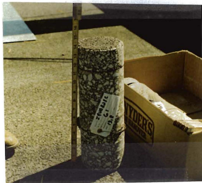
Figure 8. GPR Trace a Field Validation Core from a Thick Homogeneous HMA Pavement.
