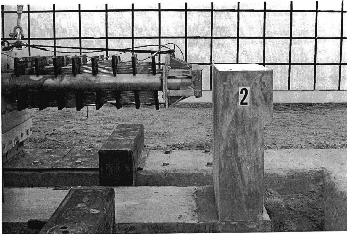
Figure 2. Specimen and Pendulum Setup.
