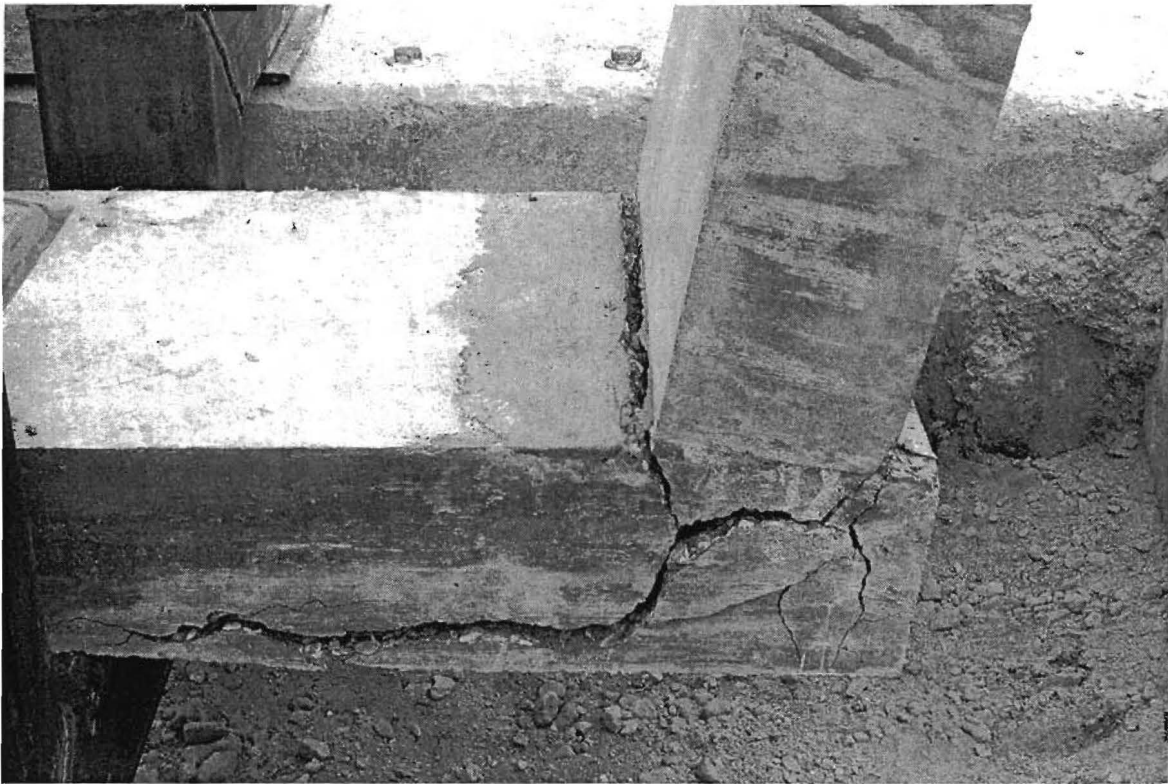
Figure 6. Steel-Reinforced Specimen, Single Impact Loading.
