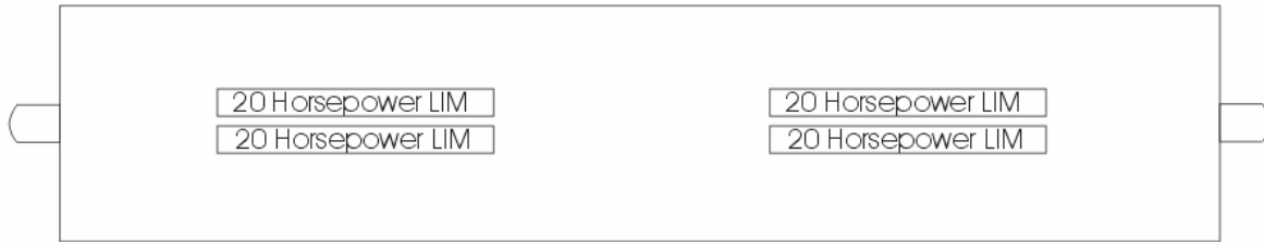
Figure 2.9. Arrangement of Linear Induction Motors Under the Frame of an MTM.
