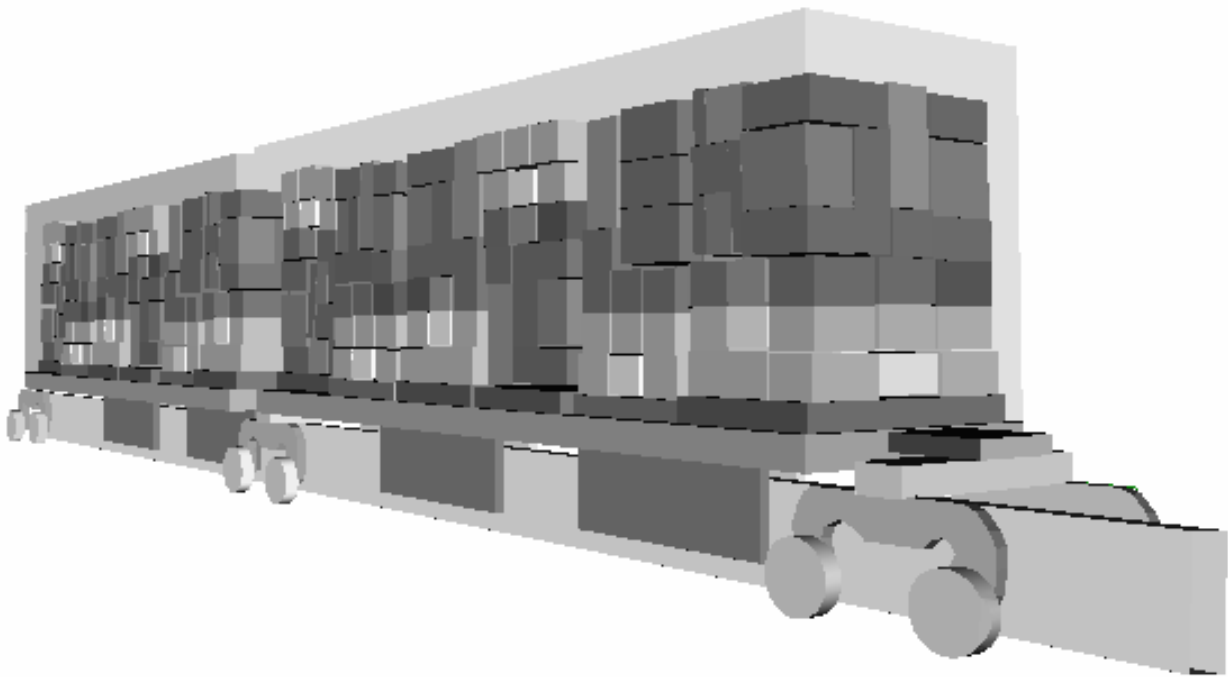
Figure 2.7. Positioning of Wheel Assemblies, Motors, and Cargo of Linked MTM Cars.
