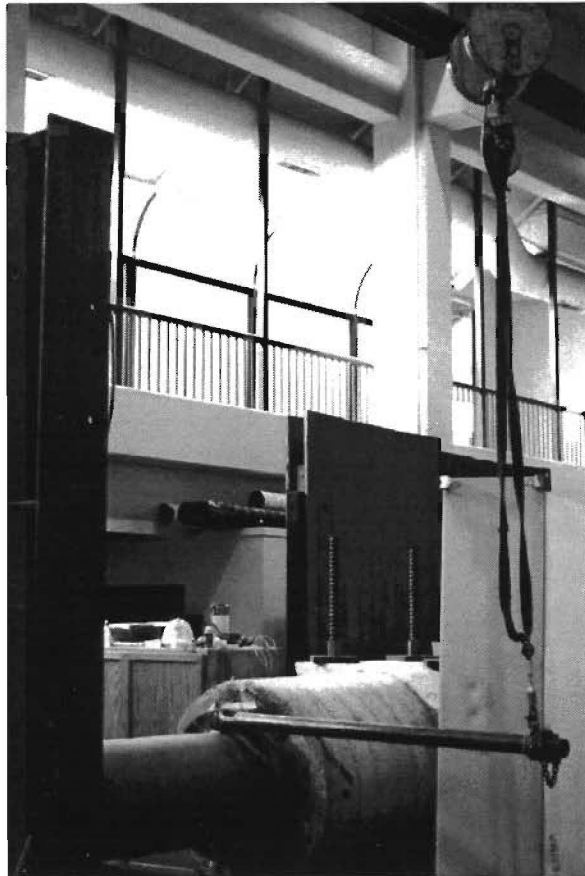
FIGURE 50 Photograph illustrating apparatus for measuring tightening torque.
