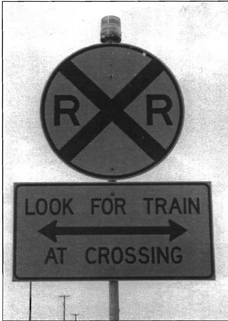
Figure 2.4. Strobe Light and Supplemental Sign Enhancement
