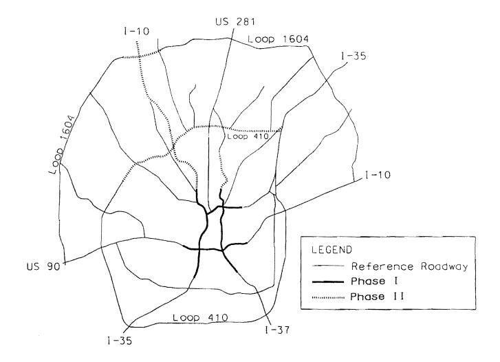
Figure 2. Existing and Future (1996/1997) Components of TransGuide System
