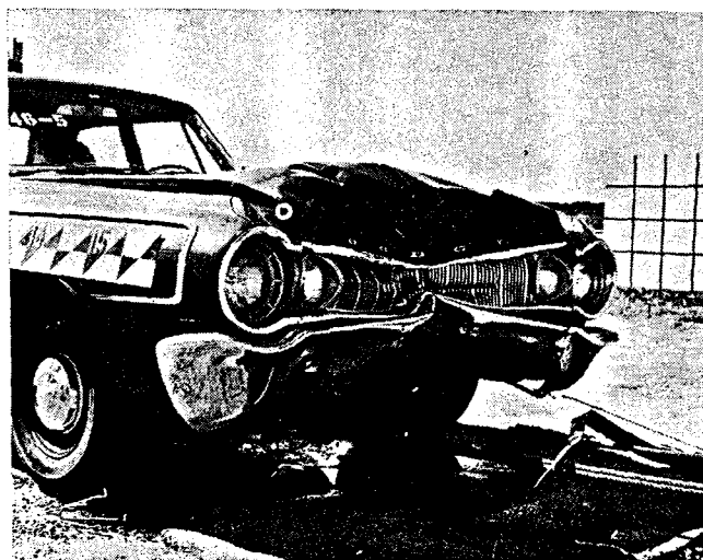
Figure 40. Damaged area of vehicle after test (1146-5).
