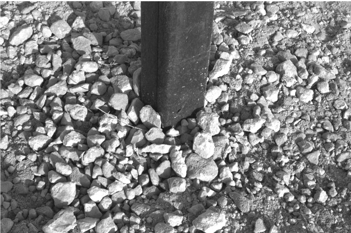
Figure 18. Recycled Plastic Sign Support Before Test 414587-3.
