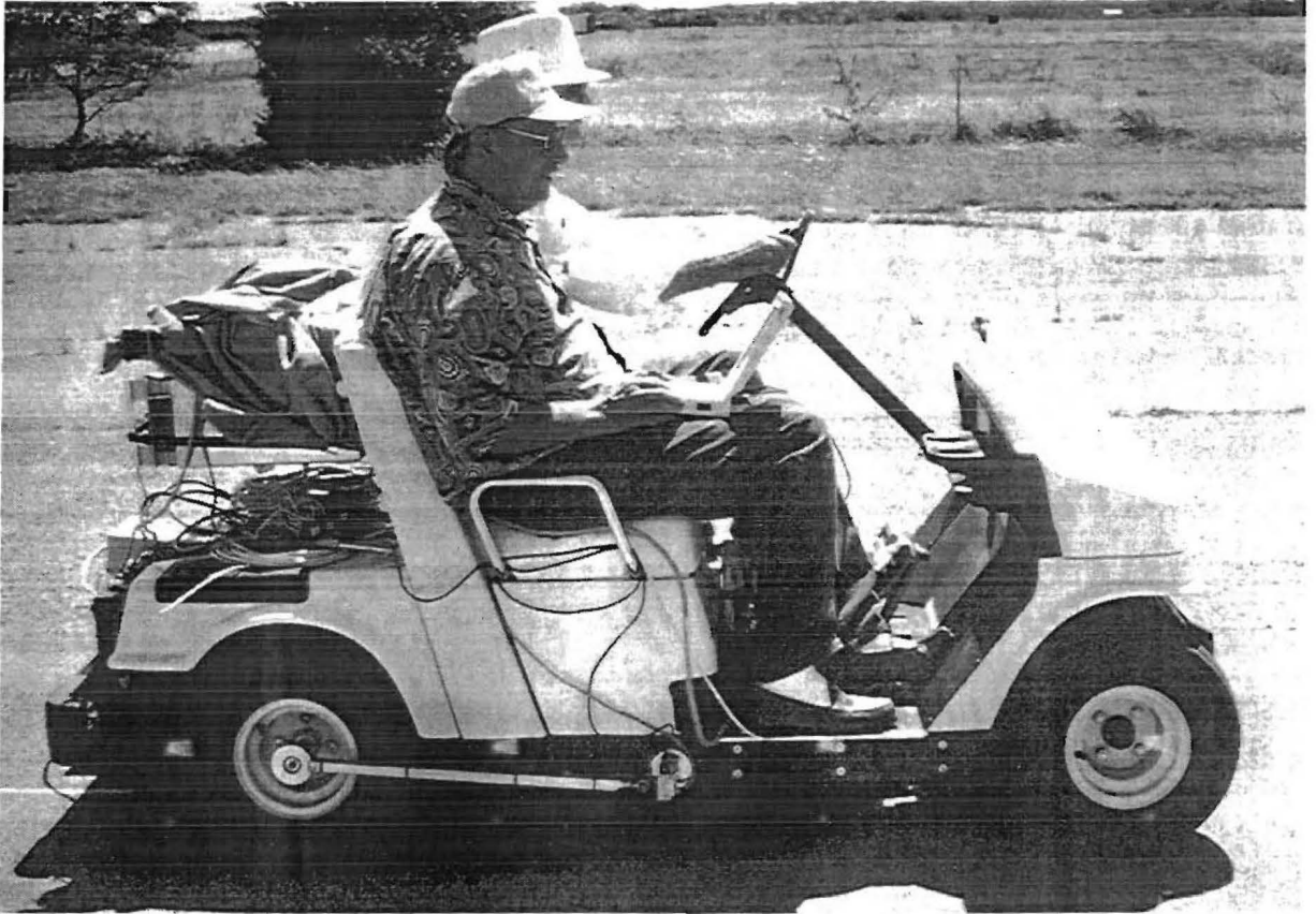
Figure 8. The Construction Profiler Developed by TxDOT.
