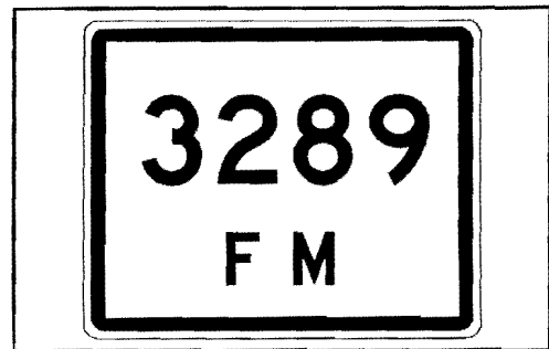
Figure IV-14. Recommended Design for F.M. Route Marker
