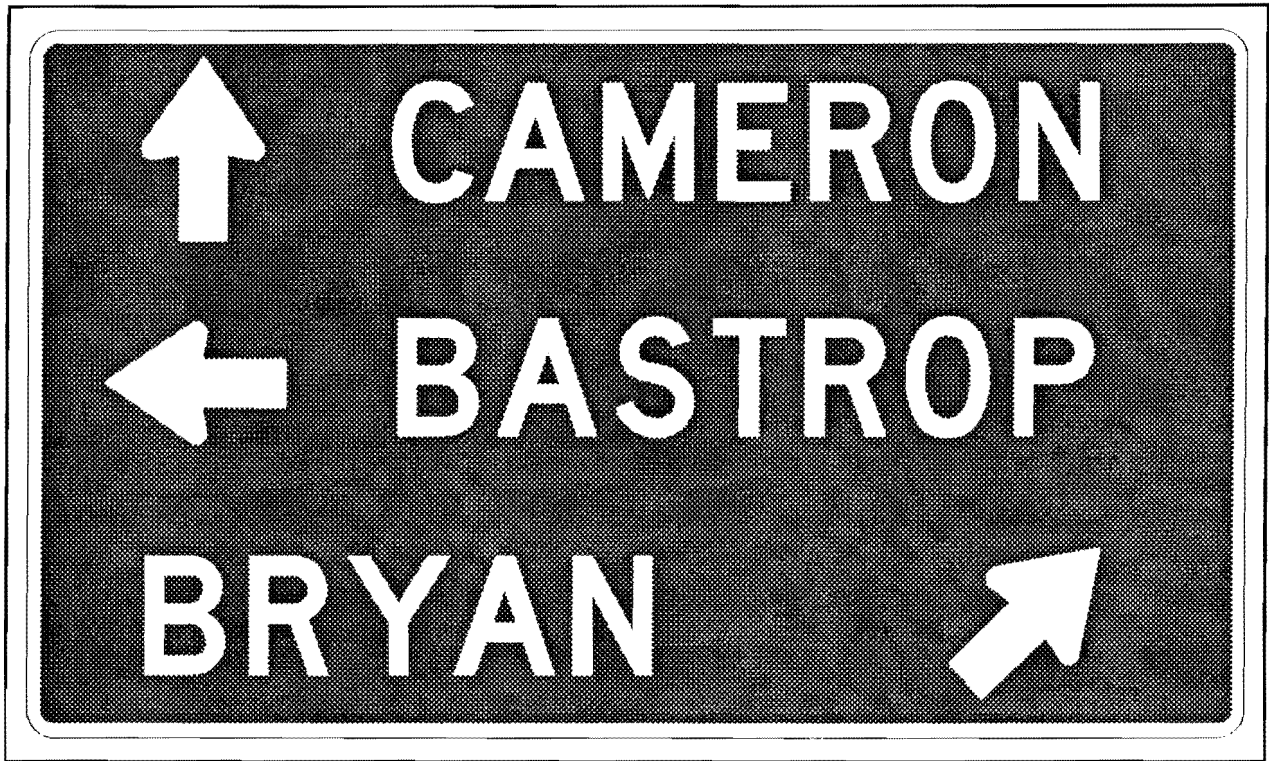
Figure VI-4. Proposed Destination Sign for a Highway Intersection with Turning Roadways - Use of Straight Arrow
