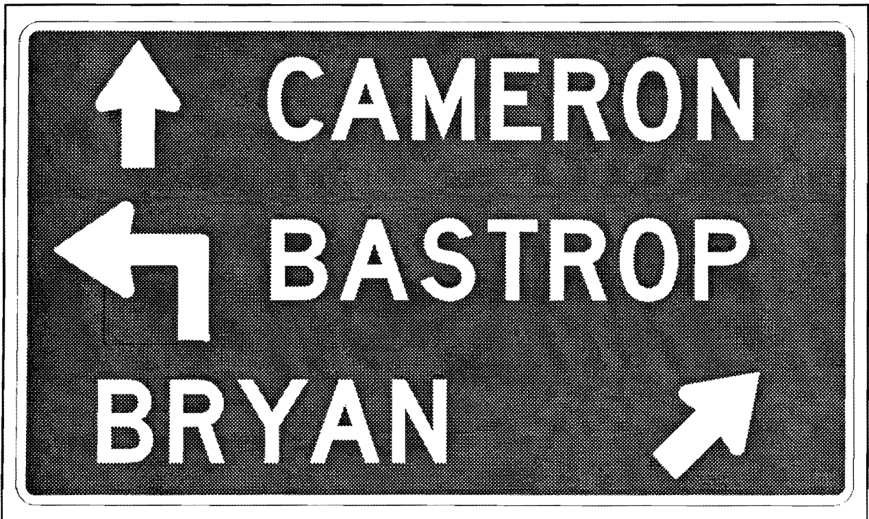
Figure VI-5. Proposed Destination Sign for a Highway Intersection with Turning Roadways - Use of Bent Arrow
