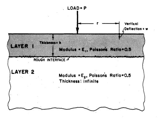
Figure 1: Two Layer Elastic System
