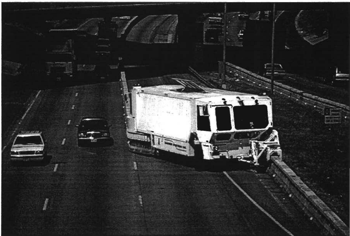
Figure 44. Machine Used to Shift Moveable Concrete Barrier on East R.L. Thornton
