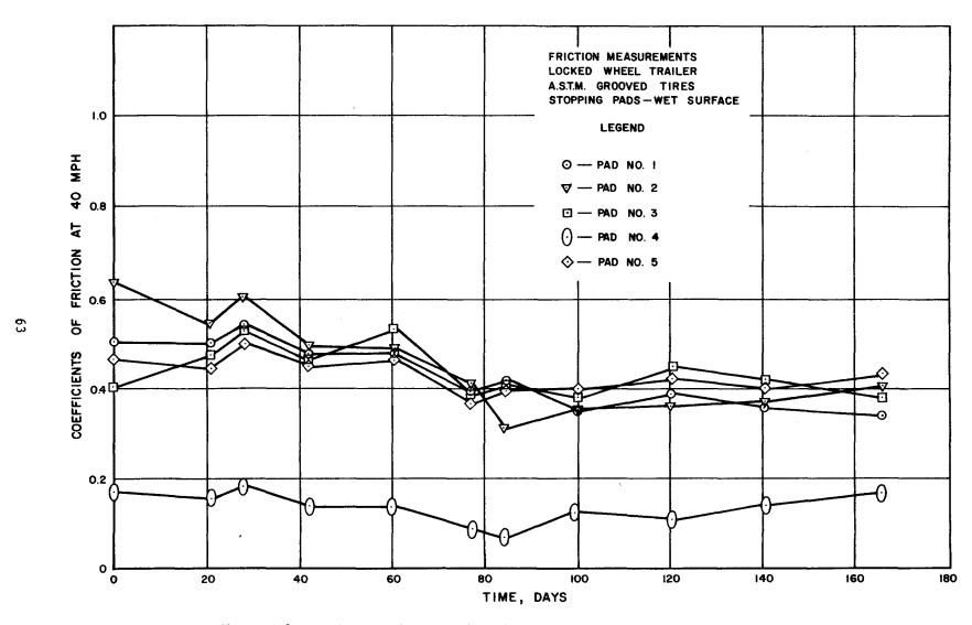
Figure C-2 - Variation of Test Pad Coefficients Over the Period of Testing.
