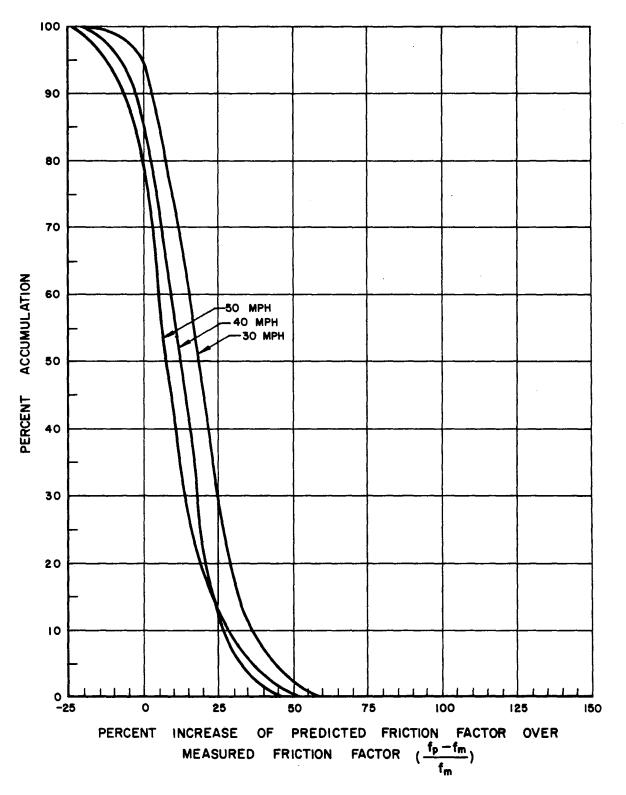
Figure C-6 - Percentile Distribution of Percent Deviation Between Measured and Computed Friction Factors Classified by Test Speed.
