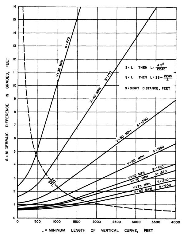
Figure 12 - Relationship Between Stopping Sight Distance and Length of Vertical Curve for Head-on Collision Criterion for 3.75-Foot Eye Height and Two-Foot Objective Height.
