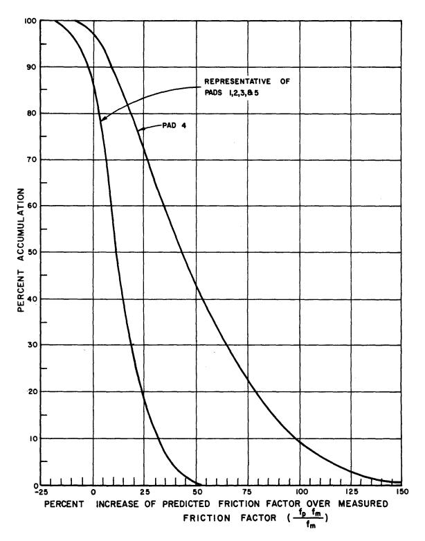
Figure C-8 - Percentile Distribution of Percent Deviation Between Measured and Computed Friction Factors Classified by Pad Number.
