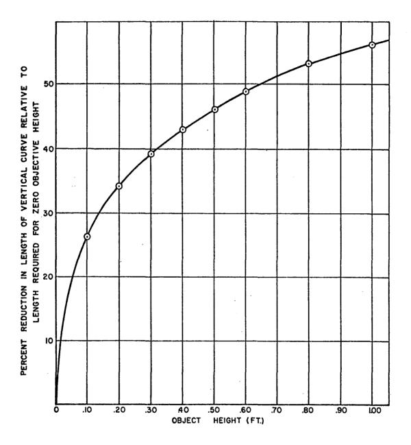
Figure 11 - Relation Between Object Height and Required Length of Crest Vertical Curve for AASHO Policy Stopping Sight Distance Standards (2).
