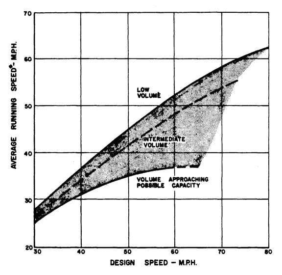
RUNNING SPEED IS THE SPEED (OF AN INDIVIDUAL VEHICLE) OVER A SPECIFIED SECTION OF HIGHWAY, BEING DIVIDED BY RUNNING TIME.
