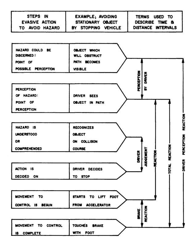
Figure 7 - The Perception-Reaction Process (13).
