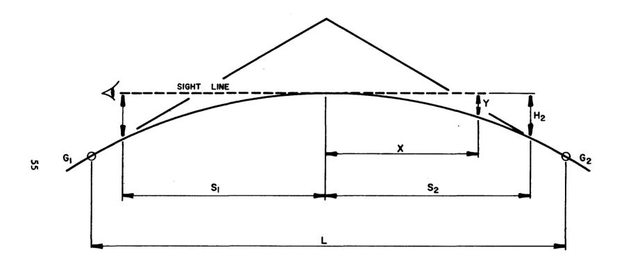
Figure B-2 - Sight Distance Configuration for S<L.
