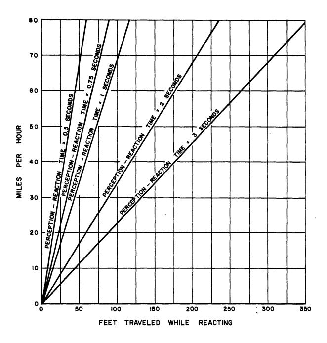
Figure 8 - Distance Traveled During Various Perception-Reaction Times for Various Speeds.
