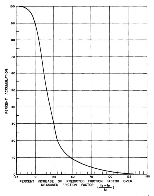
Figure C-5 - Percentile Distribution of Percent Deviation Between Measured and Computed Friction Factors for All Tests.
