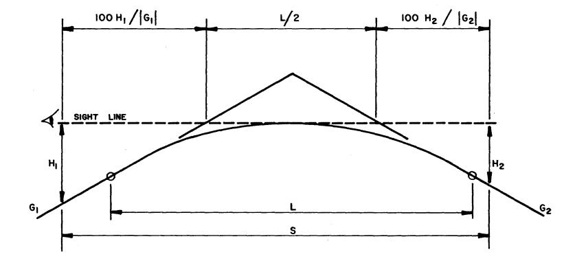
Figure B-1 - Sight Distance Configuration for S>L.
