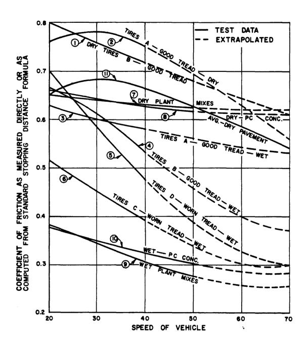
Figure 1 - Relationships Between Friction Factor and Speed for Several Conditions - AASHO Policy (2).
