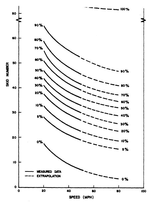
Figure 9 - Percentile Distribution of Skid Number Versus Speed Relationship for 500 Pavements in One State (14).
