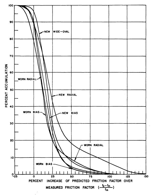
Figure C-7 - Percentile Distribution of Percent Deviation Between Measured and Computed Friction Factors Classified by Tire Type.
