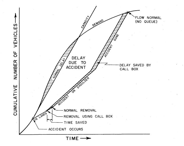
FIGURE 9. RELATIONSHIP OF FLOW CAPACITY AND DELAY.
