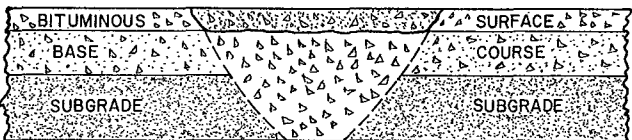
3. (A) SEAL COARSE AGGREGATE AND TACK EDGES. (B) COMPACT COLD MIX TO CONFORM WITH SURFACE GRADE. (C) SEAL OR WATERPROOF SURFACE DURING SEASONS OF RAINY WEATHER.
