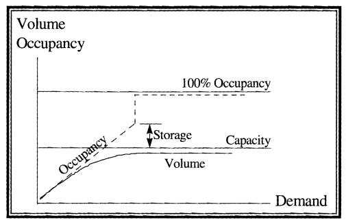
Figure 14. Volume/Occupancy Versus Demand Curve for a Signalized Approach Lane with a System Detector
