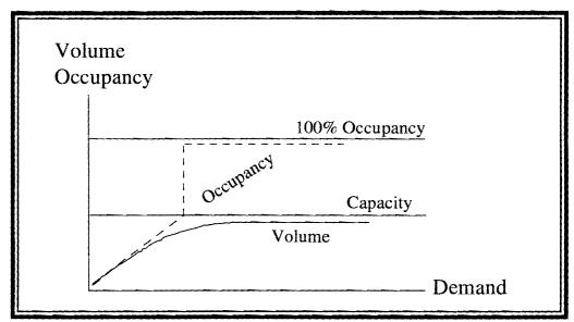
Figure 13. Volume/Occupancy Versus Demand Curve for a Signalized Approach Lane with a Stop-Bar Detector
