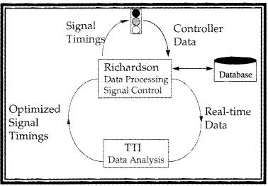
Figure 16. Data Flow between Richardson and TTI
