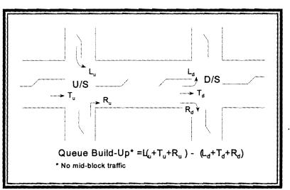
Figure 18. Input-Output Analysis on a Link
