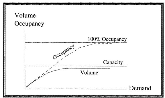
Figure 11. Volume/Occupancy Versus Demand Curve for an Uninterrupted Lane
