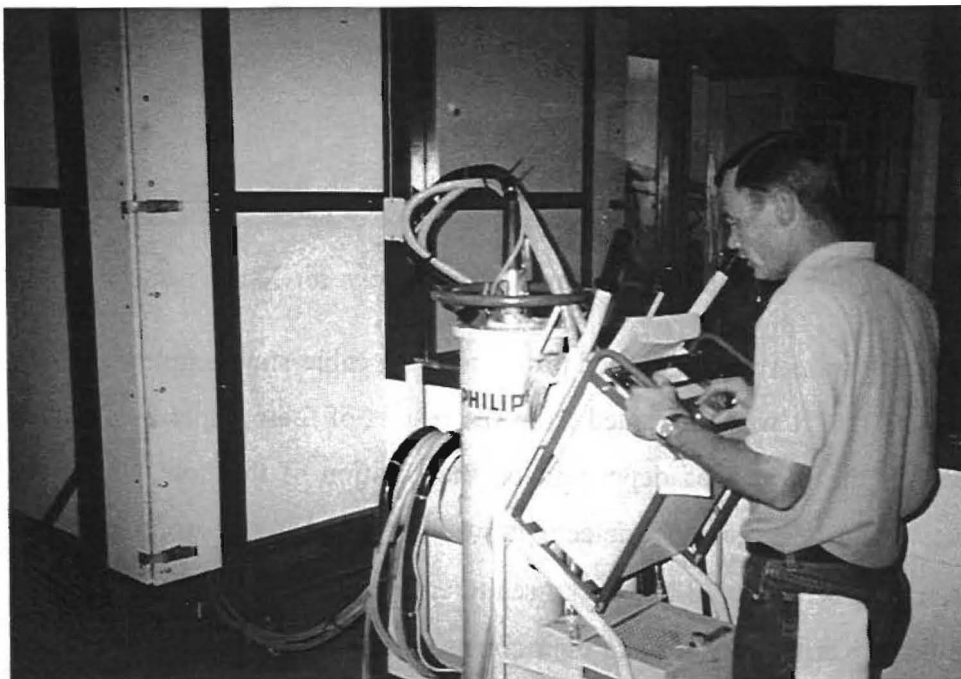
Figure 15. X-ray inspection of cable-stay specimens.
