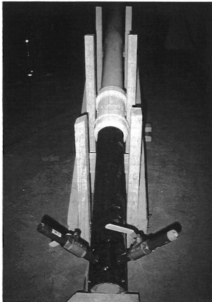
Figure 39. Inclined cable-stay sample after grouting.
