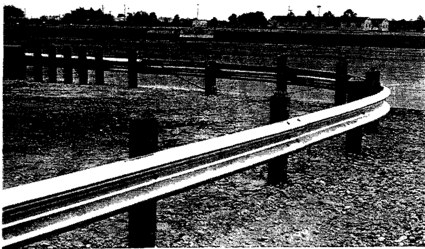
FIGURE F-91. Short Radius Guardrail before Test 1263-6
