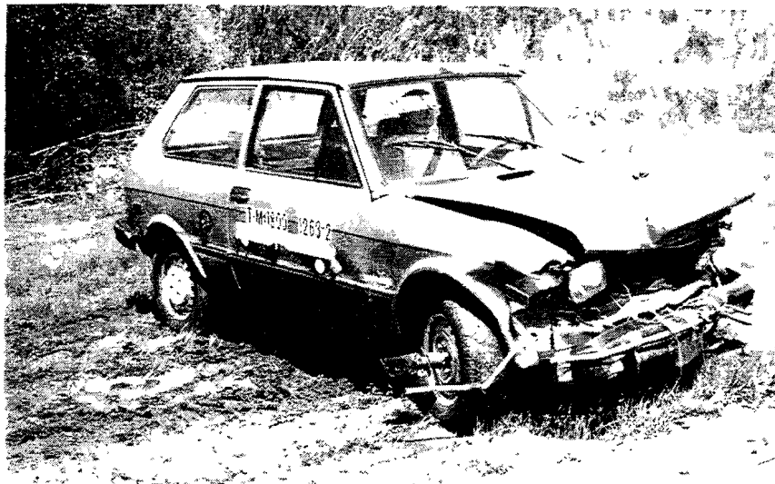
FIGURE F-32. Vehicle after Test 1263-2
