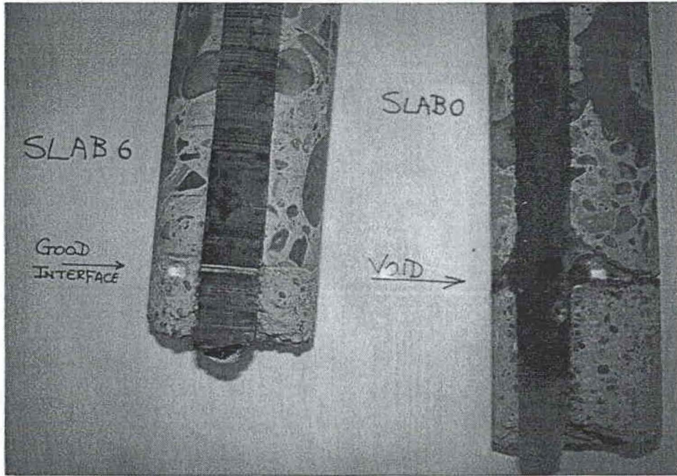
Figure 34. Results of Epoxy Core Test.
