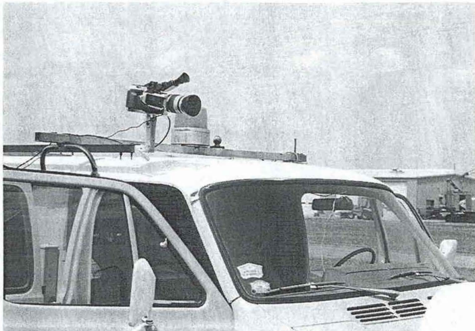
Figure 8. Video Acquisition System (DMI Information Added as a Header to the Video Image).
