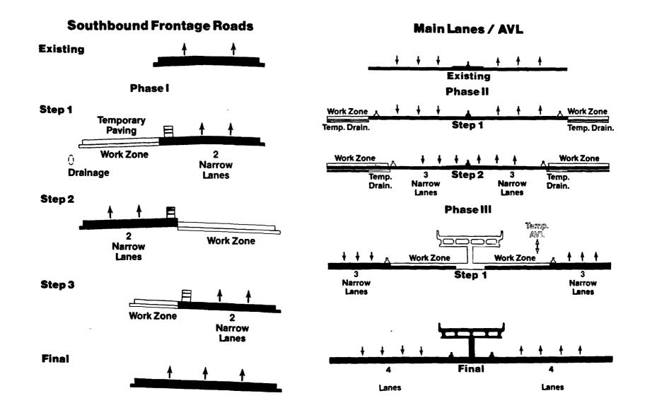
Figure 5. Typical Construction Sequencing for the US-59 Southwest Freeway Reconstruction Project in Houston
