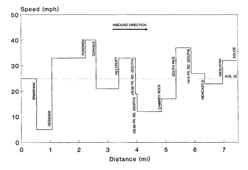
Figure 4. A.M. Peak-Hour, Peak-Direction Speed Profile for Westpark
