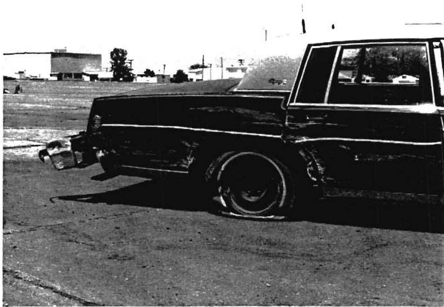
Figure 16. Damage to right side of vehicle, test 1185-6.
