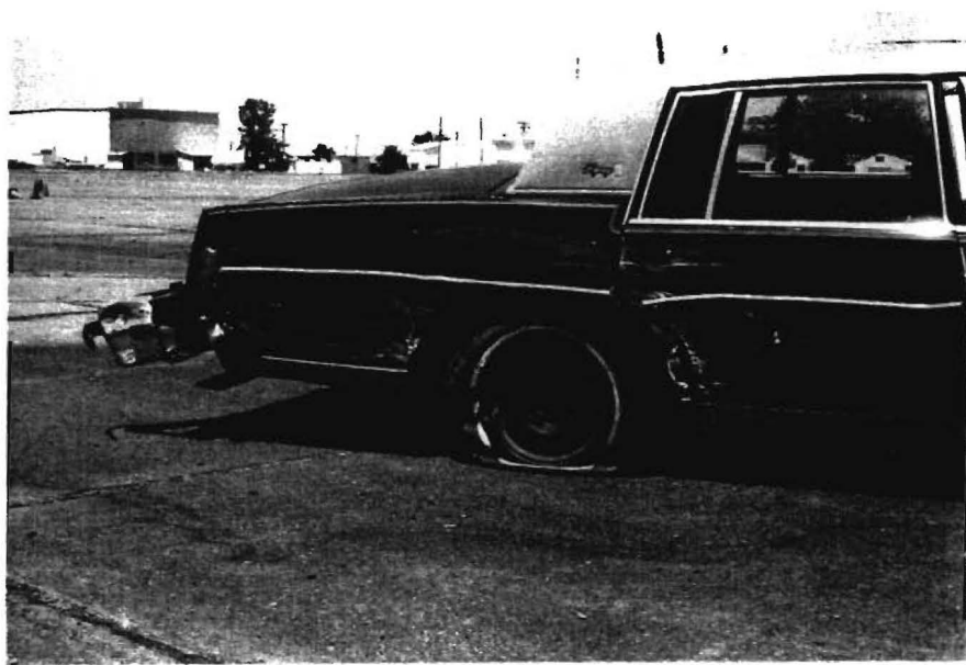
Figure 16. Damage to right side of vehicle, test 1185-6.
