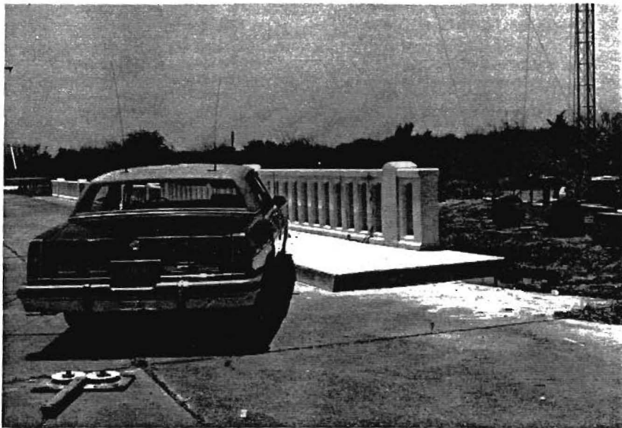
Figure 14. Vehicle/bridge rail installation geometrics for test 1185-6.
