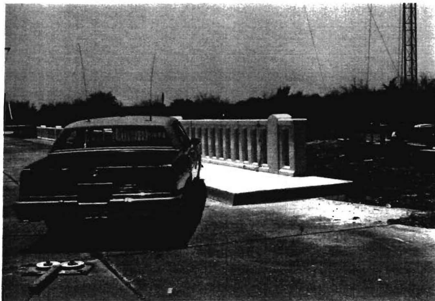
Figure 14. Vehicle/bridge rail installation geometrics for test 1185-6.
