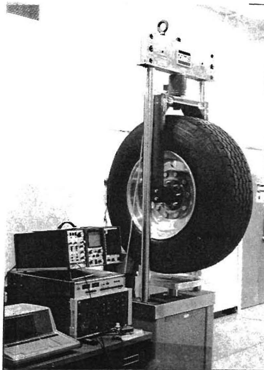
Figure 1. Wide base tire mounted in the MTS testing machine.
