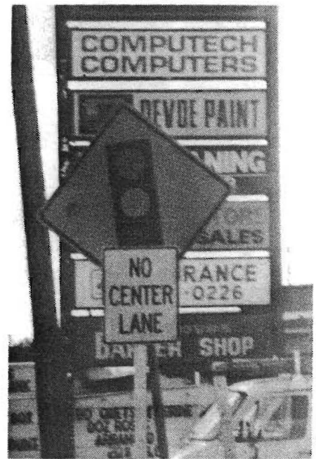
E. Field Placement of NO CENTER LANE Sign
