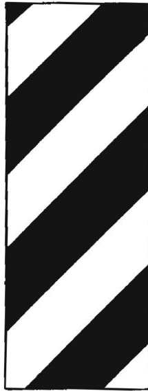
Figure D-22. Vertical Construction Panel
