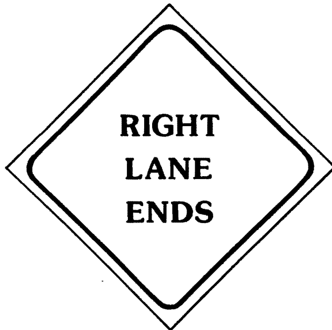
Figure D-20. Right Lane Ends Sign
