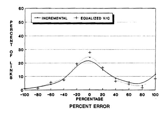
FIGURE D-8 Volume and Percent Error Distributions of Link Differences by Error Ranges for the Project Area.
