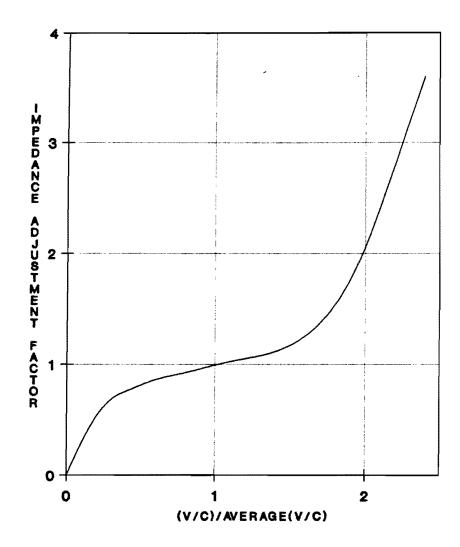
FIGURE 2 New Impedance Adjustment Function.
