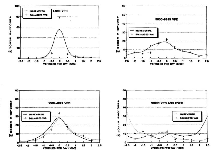
FIGURE D-9 Distributions of Link Difference by Error Range of Volume Group for the Tyler Network.
