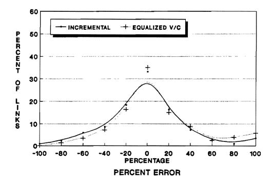
FIGURE D-7 Volume and Percent Error Distribution of Link Differences by Error Ranges for the Tyler Network.
