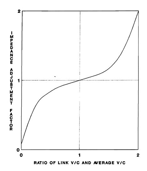
FIGURE 1 Expected Shape of Impedance Adjustment Function.
