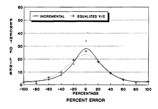
FIGURE D-3 Volume and Percent Error Distributions of Link Differences by Error Ranges for the Project Area.
