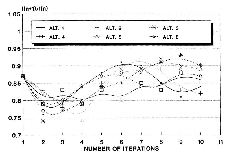
FIGURE B-7 Average V/C Ratio Changes between Iterations.
