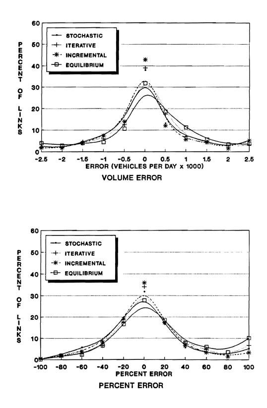
FIGURE A-6 Volume and Percent Error Distributions of Link Differences by Error Ranges for Total Network.
