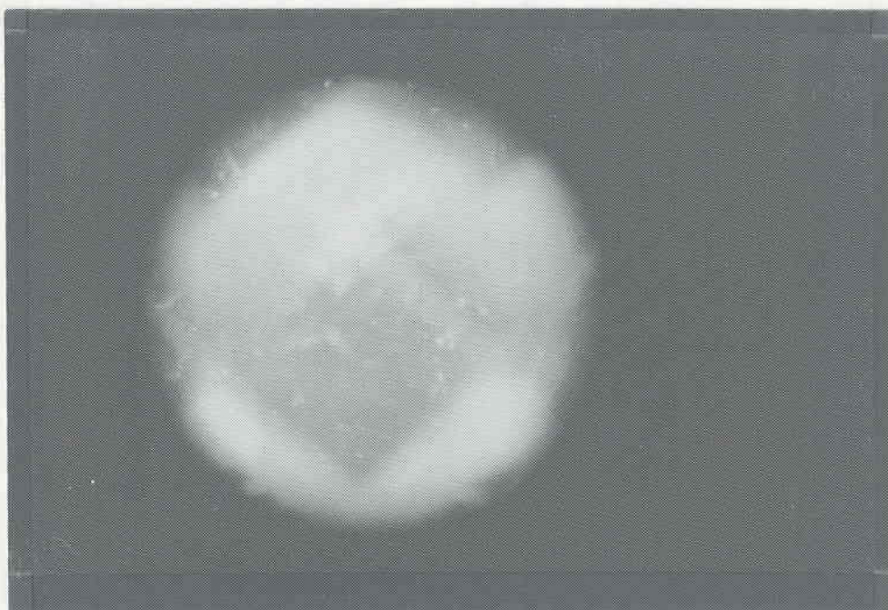
Figure 5-17. Photomicrograph of glass-faced Model 911 RPM (ID# 37) after 4400 tire impacts.
