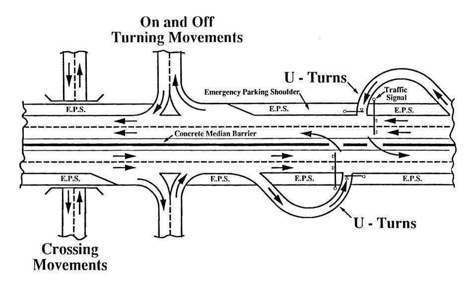
Figure 6. Separation of turning and crossing movements.
