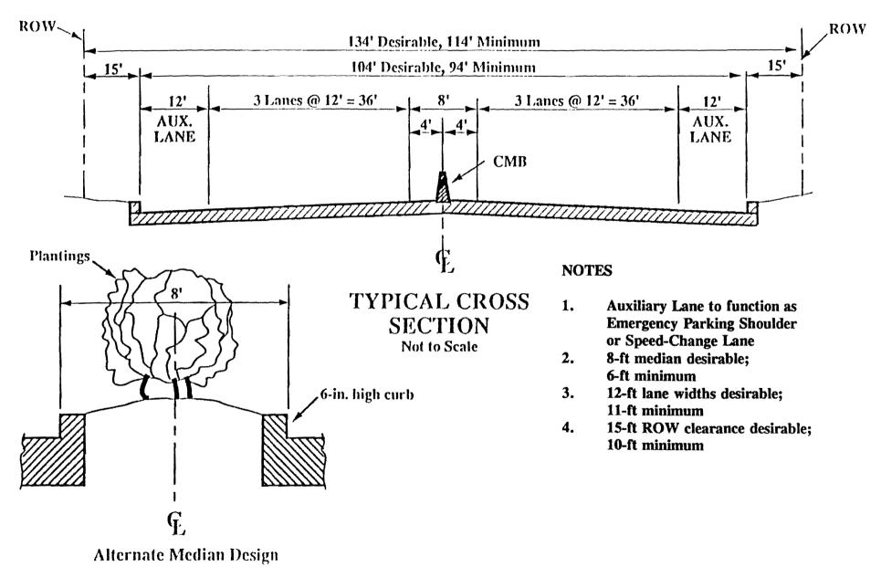
Figure 4. Proposed typical cross section.
