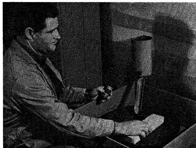
Figure 5. Grinding the exposed surface with silicon carbide abrasive.
