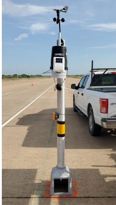
Figure 8. Leddar™ IS16 Sensor and Weather Station.
