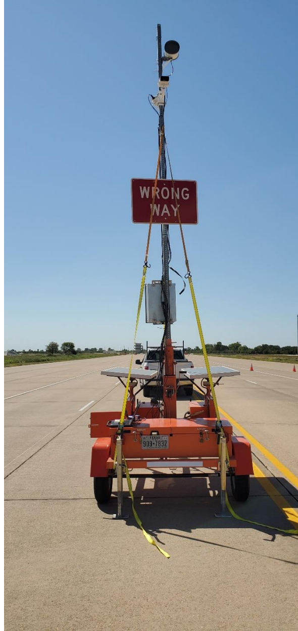
Figure 17. Carmanah® Equipment on Portable Trailer.
