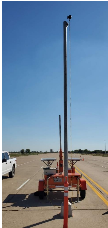
Figure 26. FLIR Equipment on Portable Trailer.
